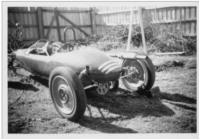
cylinder. The chassis used small-diameter tubing snugly fitted inside an alloy shell made from a Gloster Meteor drop tank.
