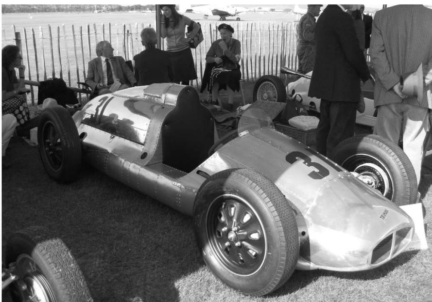
frame chassis 15-inch alloy composite wheels and transverse-leaf suspension, and ran at some sprints and hillclimbs. It too has lost its Vincent engine, but it now has a 650 Triumph. More details in the classifieds.
